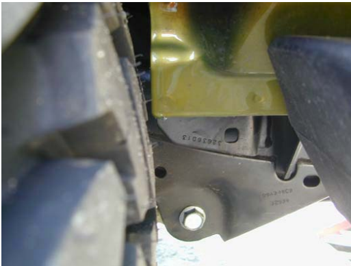
Above – No cutting, vehicle fully flexed - 3.5 lift kit, 35x12.5 Toyo's Above – Fender trimmed, vehicle on level ground - 4.5 lift kit, 37x13.5 Toyo's
