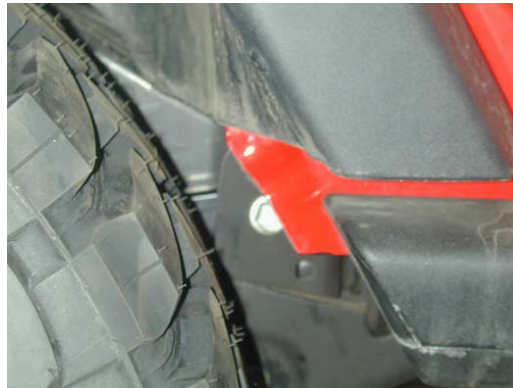
Above – No cutting, vehicle fully flexed - 3.5 lift kit, 35x12.5 Toyo's Above – Fender trimmed, vehicle on level ground - 4.5 lift kit, 37x13.5 Toyo's
